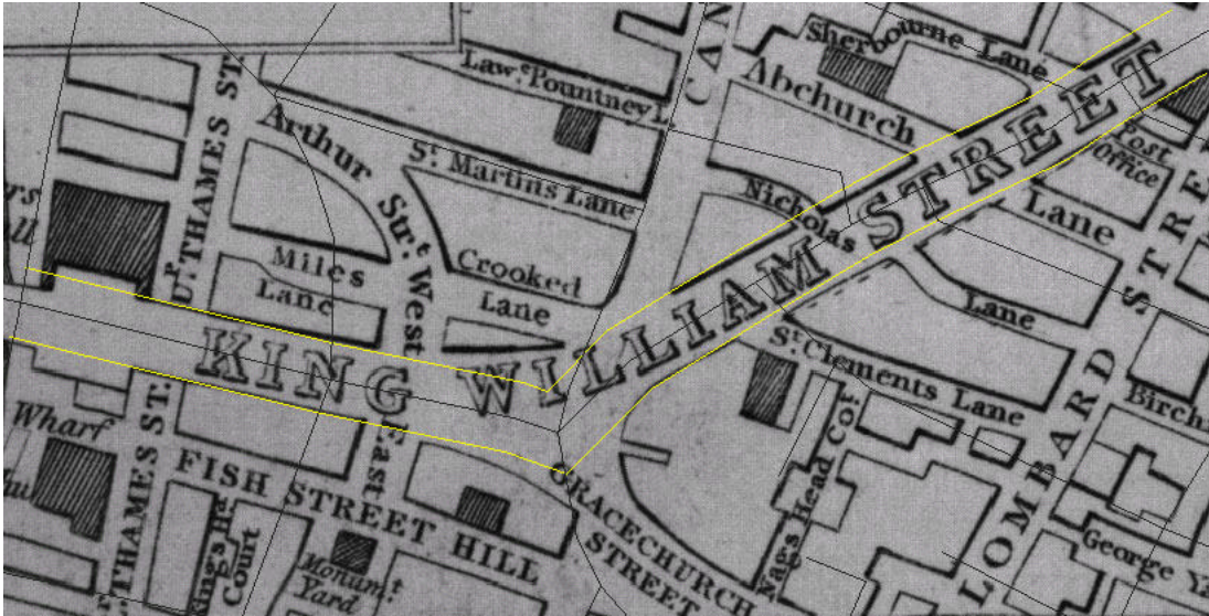
Figure 4. CAD file showing modern georeferenced streets and “frontage lines” overlaid on Tallis’ map detail
