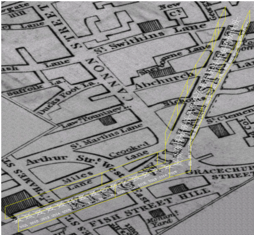
Figure 5. CAD file showing digital model of King William Street with extruded “frontage lines” and virtual camera positions overlaid on Tallis’ map detail
